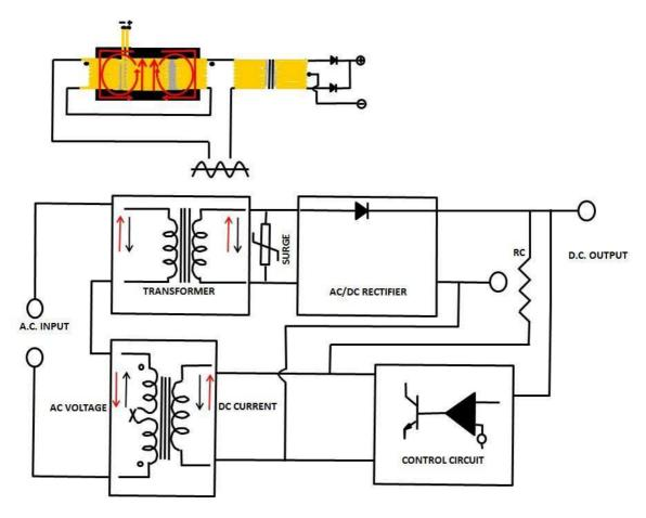
The nature of the primary magnetic amplifier is inductive; this produces lower input power factors in mag-amp designs compared to other technologies. The input current harmonic distortion is typically less than 10% and the output efficiency is approximately 70% for single phase designs and 85% for three phase designs.
