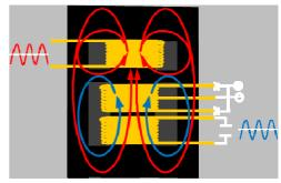
The secondary of the ferroresonant transformer consists of a tank circuit that is resonated by a high voltage winding and capacitors. This capacitor tank circuit keeps the magnetic flux of the secondary winding in saturation. The effect of the saturated secondary is inherent voltage regulation (an open feedback loop regulator) and the loads on the secondary are not linearly reflected back to the primary.
