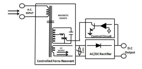
The characteristics of a saturated secondary and physical separation between the primary and secondary windings in the power transformer design also provide excellent attenuation to incoming transient voltages that may be present on the AC line.
